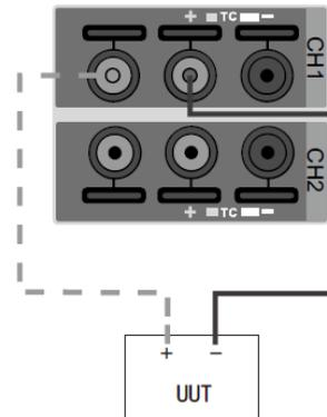
Figure 5 Connection way of Electric Current(mA) Measurement
